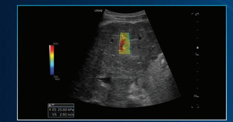
Liver 2D Shear Wave Elastography, C1-6-D
